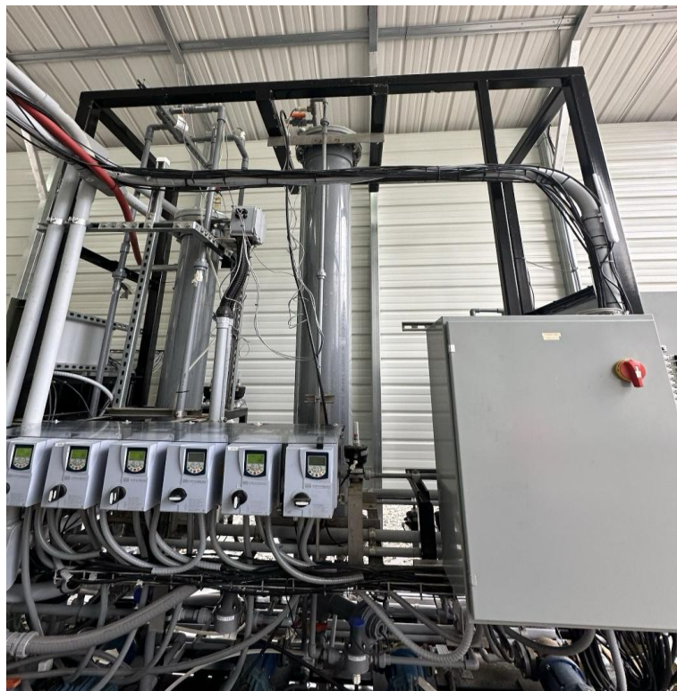
Figure 13-5: LSS Column at the Pilot Plant
