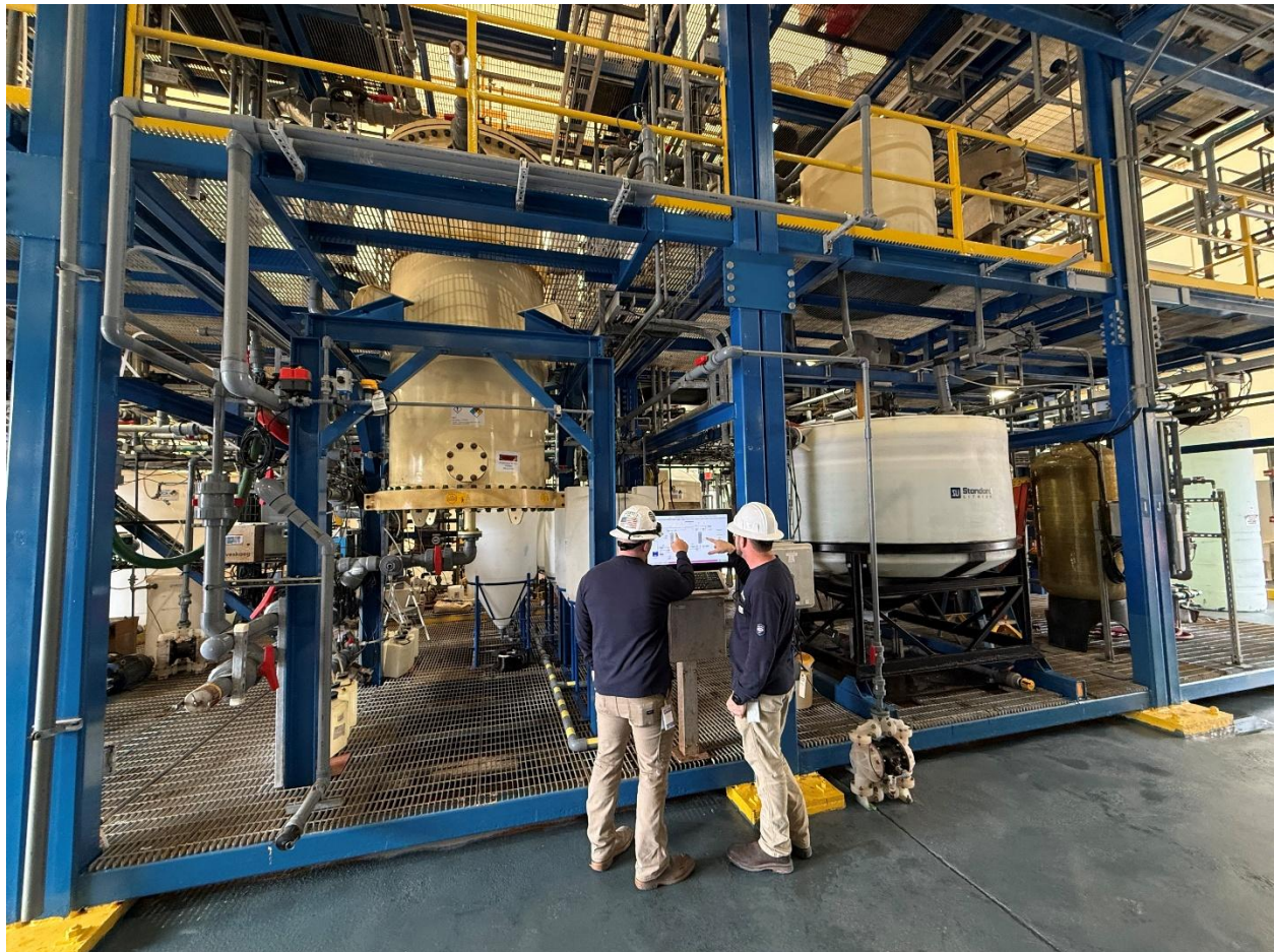
Figure 1: Operators at control panel in front of commercial-scale (8' x 4') DLE column at Standard Lithium's Demonstration Plant near El Dorado, Arkansas.
