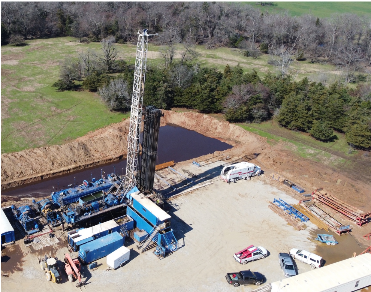
Figure 1: Drill rig at the new borehole/well location in East Texas. The drill rig has since demobilized from this location and has been replaced by a workover rig to complete perforations, final testwork and sampling.
